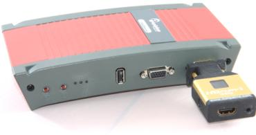
4. Connect the audio cable from HD Fury 2 to the line-in (and not the microphone) port of the Experiment Center PC.
